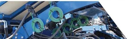
METERING TUBE is used in place of a traditional orifice to provide even distribution to each row. In a typical in-furrow application scenario a 0.030" orifice is replaced with an 8' length of metering tube having a passageway of 0.096". The combination of length and diameter equalizes flow to each row. Metering tube virtually eliminates the problem of plugged orifices.
