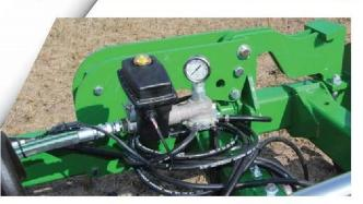
The Torpedo™ cooler is the central piece of the SureFire Anhydrous Ammonia Application System. It is a high capacity, extremely accurate, efficient heat exchanger. However, a cooler is only one component of an NH3 application system.
